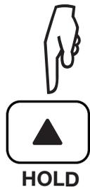
Pressing the **HOLD** key freezes the display of the measurement. This can be done in all functions except voltage in the **MΩ** setting.
