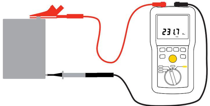
The instrument displays the voltage on the terminals. It detects whether the voltage is AC or DC and, if it is AC, displays its frequency.
