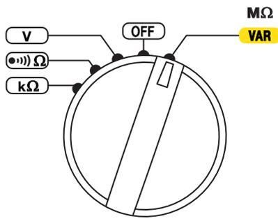
Set the switch to the **MΩ** position.
