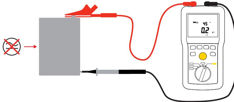
Use the leads to connect the device to be tested to the terminals of the instrument. The device to be tested must not be live.
