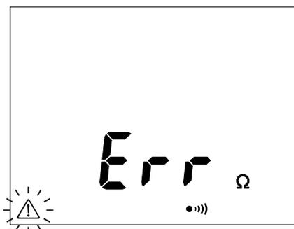
If, during a continuity or resistance measurement, the instrument detects an external voltage in excess of 15 V (AC or DC), it interrupts the measurement and displays the screen shown opposite.
