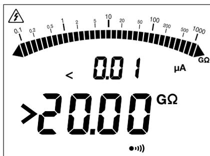
If, during an insulation measurement, the value to be measured exceeds the measurement range (which depends on the test voltage), the instrument so reports.
