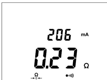
The instrument makes the measurement directly. It displays the result and the measurement current.
