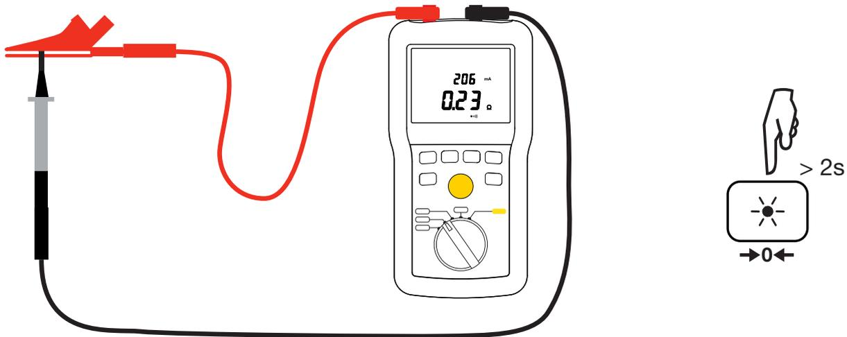
The display changes to zero and the  $\rightarrow 0 \leftarrow$  symbol is displayed. The resistance of the leads will be systematically subtracted from all continuity measurements. If the resistance of the leads is  $> 10 \Omega$ , there is no compensation.
