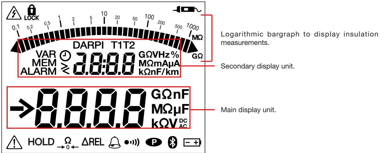
When the measured value is below the minimum, the instrument displays - - - - .
