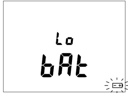
The batteries must then be replaced (see § 4.2)), since the battery life indication is no longer reliable.
