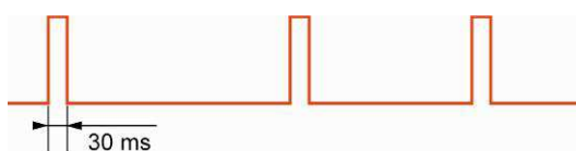
Example of pulse train timing in pulse mode
