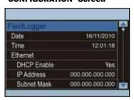
Data logger and display parameters can be changed and viewed on this screen.
