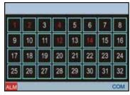
A 32-position grid where each numbered position is related to its equivalent alarm or event. When an alarm is active, its number will be displayed in red on this screen.
